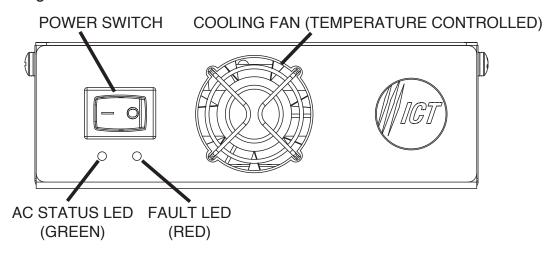
Figure 2: ICT Inverter Back Panel
