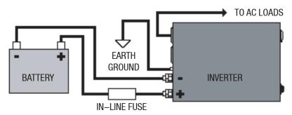
Figure 3: ICT Inverter Wiring Diagram
